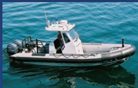
Titan 240 T-Top Overall length: 27' Beam: 9' 10" Horsepower range: 300 - 450 hp
