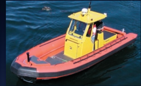
Titan 249XL Overall length: 27' Overall beam: 10' 4" Horsepower range: 300 - 450 hp
