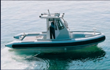
Titan 190 - Jet Overall Length: 19' Beam: 9' 4" Horsepower range: 240 - 280 hp
