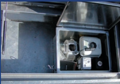
Portable pump in below deck storage
