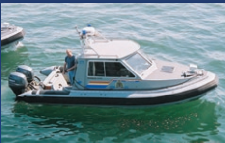
Titan 220 Pilot Overall length: 23' Beam: 9' 6" Horsepower range: 180 - 300 hp
